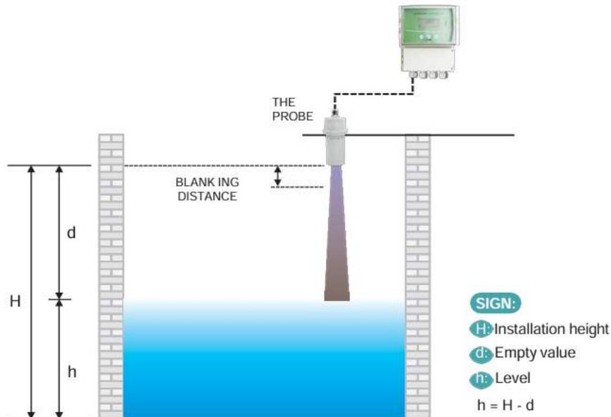
**Blind Zone:** The ultrasonic sensor cannot detect echoes at the same time when transmitting ultrasonic waves. When the probe is very close to the liquid surface, the emitted wave and the echo will overlap and cannot be distinguished. Within this area there is no explicit/ reliable measurement possible. This is blind zone (Blanking distance). During installation, the probe should be a certain distance higher than the maximum liquid level to prevent the liquid level from entering the blind zone.
