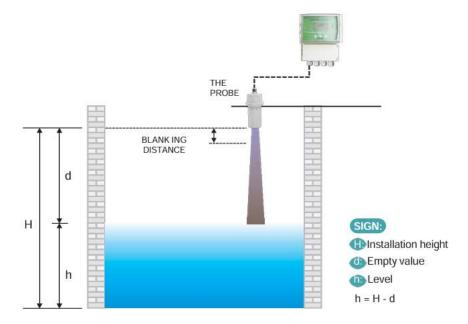
Blind Zone: The ultrasonic sensor cannot detect echoes at the same time when transmitting ultrasonic waves. When the probe is very close to the liquid surface, the emitted wave and the echo will overlap and cannot be distinguished. Within this area there is no explicit/ reliable measurement possible. This is blind zone (Blanking distance). During installation, the probe should be a certain distance higher than the maximum liquid level to prevent the liquid level from entering the blind zone.
